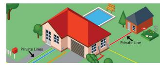
Here's one general rule: If the utility runs from the street to the meter, it will be marked up to the meter. If the utility is installed from the meter to another location on your property, it will not be marked.
